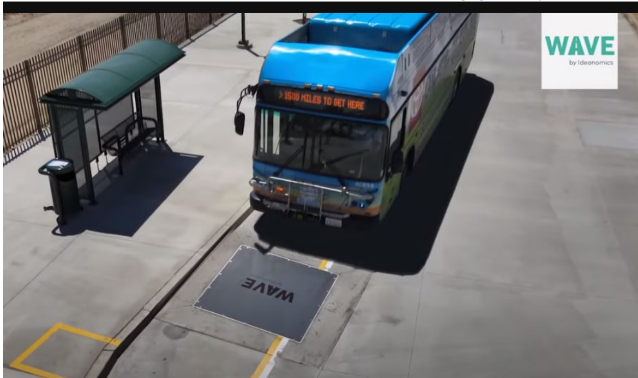
Exhibit D.4 Wireless Inductive Charging Roadway Embedded Pad
