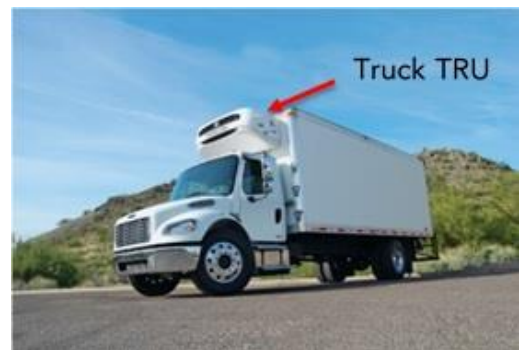
FIGURE 46: TRANSPORT REFRIGERATION UNIT MOUNTED ON TRUCK
