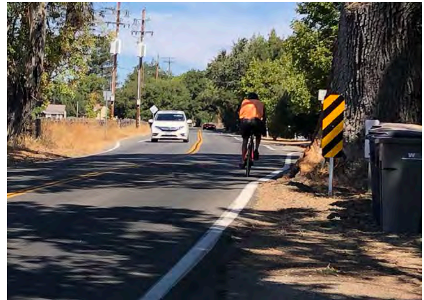
Along Alamo Pintado Road, approximately 0.2 miles south of Santa Barbara Avenue, the road narrows and the bike lanes cease. During this segment, cyclists enter a narrow lane with motorized traffic. This short interruption in an otherwise long segment of bike lanes may be enough to deter some from using the route.
