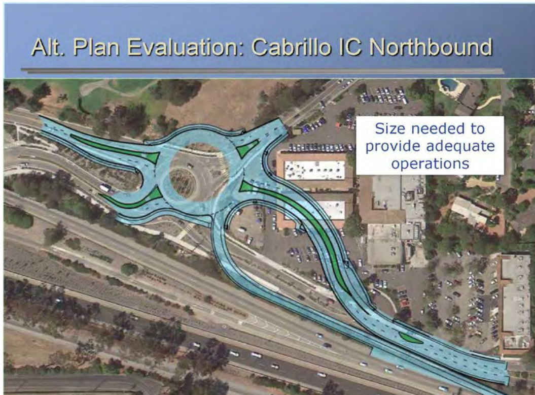
Figure 4 shows a close-up of the size of the roundabout and associated features
